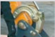
Drop forged parts used in flail head articulation
